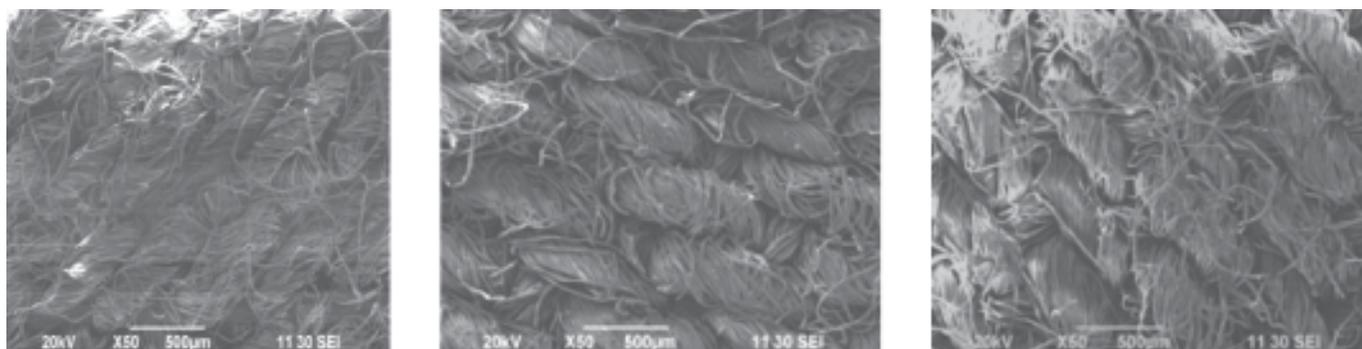
**Figure 6.** (a) Electron microscopy of jeans Bio-polished by a commercial enzyme (b) Electron microscopy of jeans with no treatment (c) Electron microscopy of jeans Bio-polished by *Trichoderma cellulase*.
