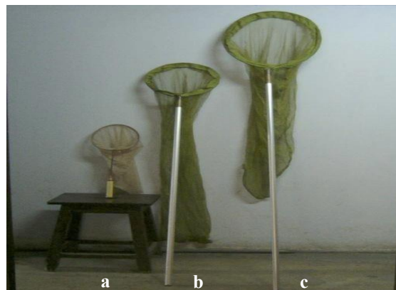
Fig. 1. Categories of insect sweeping nets of different sizes used for butterfly samplings: a. Small size insect net for capturing small butterflies available on soil surface; b. Net for capturing butterflies on herbs, shrubs and hedges at man-height level; and c. Net used for capturing butterflies on trees above man-height level.
