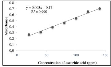
Fig. 2 Calibration curve for the determination of ascorbic acid concentration in leaf extracts.
