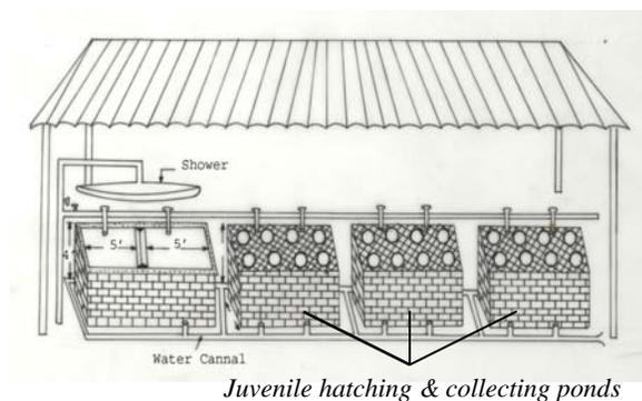
**Fig. 1a.** Induced breeding and hatching ponds with shed for commercial farming of *P. globosa*.
