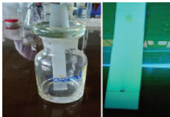
Figure 4: A) Thin layer chromatography of solasodine extract. B) TLC plate under UV light showing a single spot
