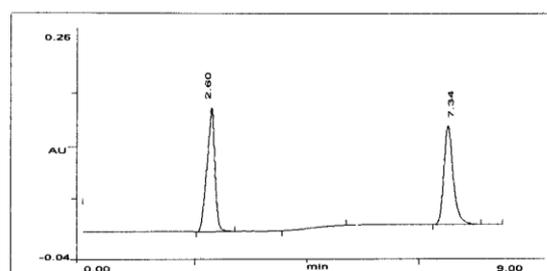
**Figure 4.** Chromatogram of Standard Rosuvastatin Calcium ( 10 µg/ ml); (Rt 2.60), and Fenofibrate ( 10 µg/ ml); (Rt 7.34) measured at 252 nm, mobile phase Acetonitrile: Methanol: Water (50:40:10).
