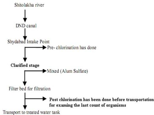
FIG 1: A schematic diagram showing the treatment procedure of supplied water.
