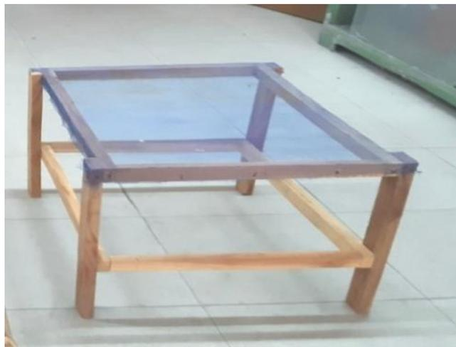
**Figure 2.** Open sun rack dryer
