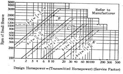
Fig. 1. Belt section from horsepower and speed
