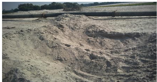
Figure 1a. River Dredged Soil (RDS) piled at riverside.
