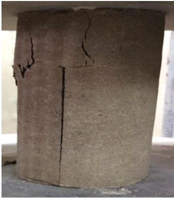
Figure 9. Typical failure pattern of the stabilized RDS-cement specimen under compression
