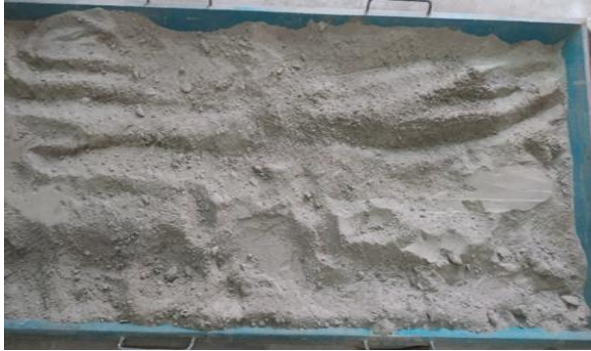
Figure 1b. River Dredged Soil (RDS) after air drying in laboratory.
