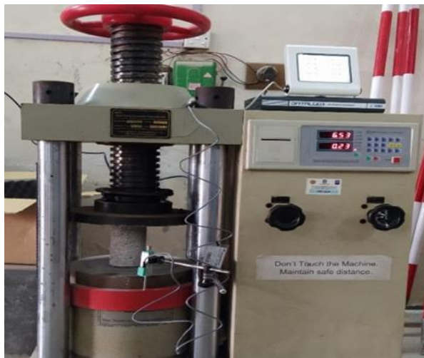
Figure 4. Test setup for unconfined compression test with data logger.
