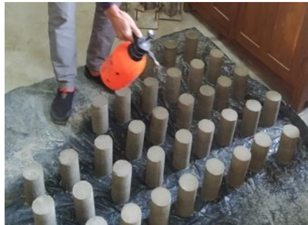
Figure 3. Curing operation using sprayer.
