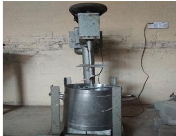
Figure 2. Mixture machine used for mixing cement with RDS.
