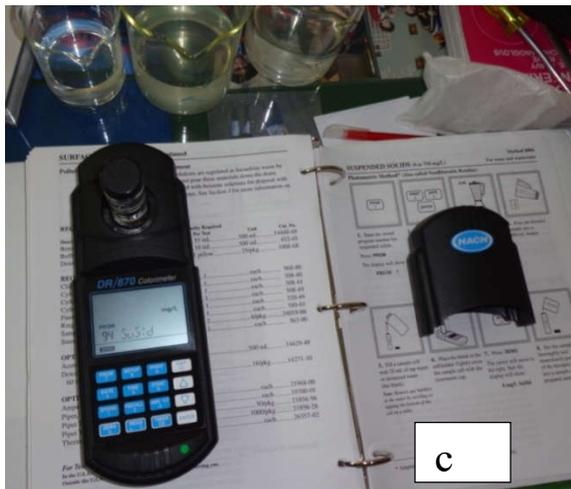
Figure 2. Measuring (a) pH and (b) Dissolved Oxygen (DO) with the Fisher scientific, Accumet XL60(c) Measuring Suspended Solids with HACH DR/870 Colorimeter.
