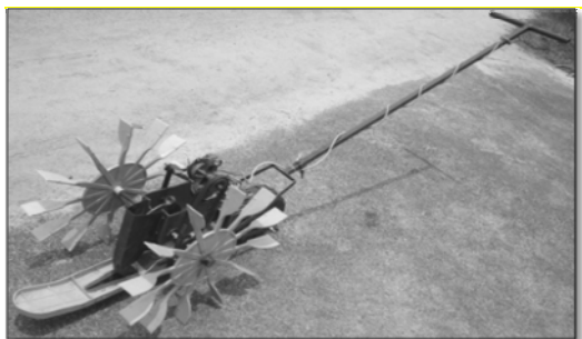
Fig. 1. Photographic view of the motor operated USG applicator
