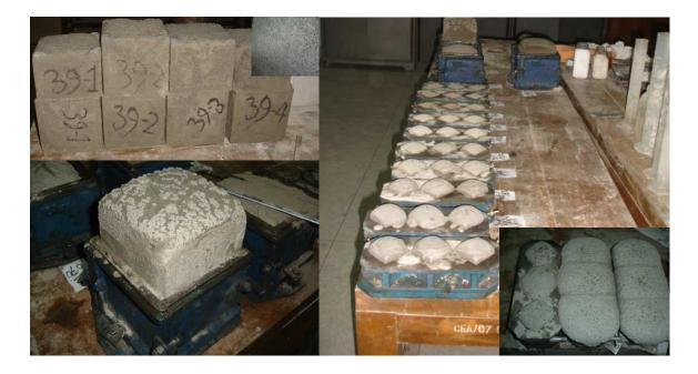
Figure 1: Volumetric expansion in cube sample and voids distribution in mortar matrix
