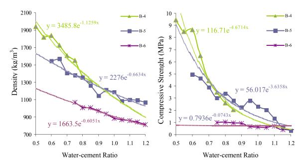
Figure 5: Comparison of Density and Compressive Strength due to increment of Volume-surface Ratio and Aluminium Content
