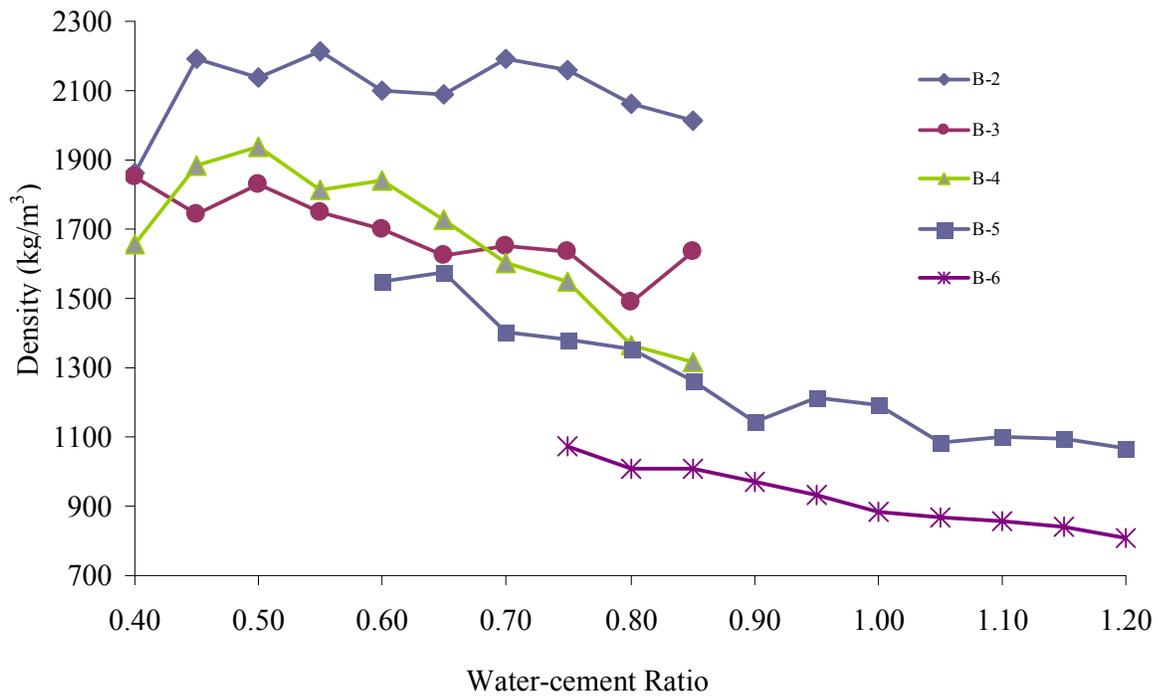
**Figure 3: Relationship between density and water cement ratio**
