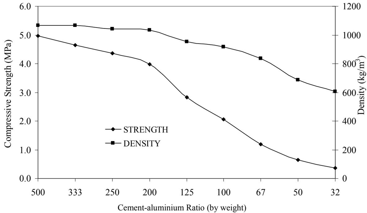
**Figure 2: Effect of Aluminium content on density and compressive strength of hardened cement (1071 kg/m<sup>3</sup>) with water (643 kg/m<sup>3</sup>)**
