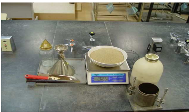
Figure 4.1: Typical arrangement of sand cone test apparatus (geotech.org)
