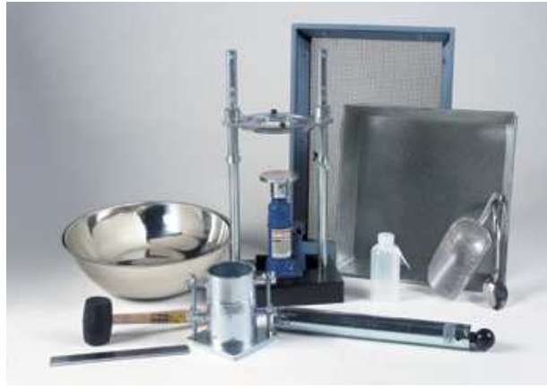
Figure 4.2: Standard proctor test apparatus (geotech.org)
