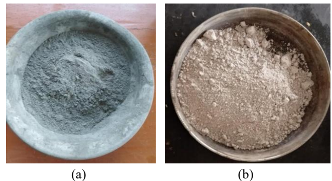
Figure 1: Concrete Ingredients: (a) Cement and (b) Limestone powder.
