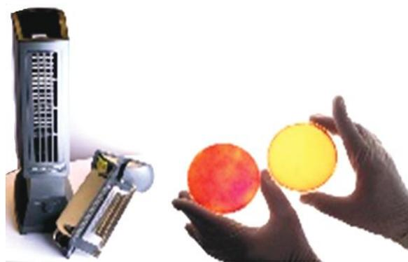
**Figure 04: Air ionizer and collection plate and the effect on the culture media on the right with no growth (source: Laboratory US department of Agriculture)**
