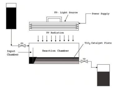
Fig. 1. Schematic diagram of the Photo-catalytic reactor.
