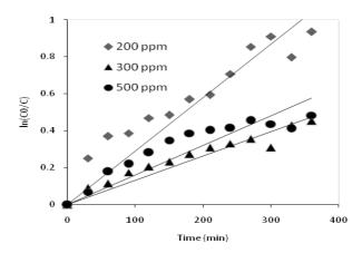
Fig. 5.  $\ln(C_o/C)$  versus time plot for RY degradation. (initial concentration,  $C_o = 200, 300, 500$  ppm; Catalyst dose = 5 g TiO<sub>2</sub> /5 g cement; Operation time = 360 min;  $T = 40^{\circ}$ C; Volume of solution = 100 ml; solution layer thickness =3.7mm).
