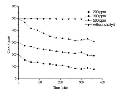
Fig. 3. Effect of different initial RY concentation on photodegradation. ( $C_o = 200, 300, 500$  ppm; Catalyst dose = 5 g TiO<sub>2</sub> /5 g cement; Irradiation time = 360 min; T= 40°C; Solution layer thickness = 3.7 mm)
