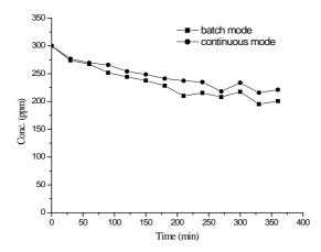
Fig. 8. Comparison of photocatalytic degradation of RY between continuous and batch mode at constant initial solution concentration and solution depth. ( $C_o = 300$  ppm; Catalyst dose = 5 g TiO<sub>2</sub> /5 g cement; Irradiation time = 360 min;  $T = 40^{\circ}$ C; Solution layer thickness = 3.7 mm.)
