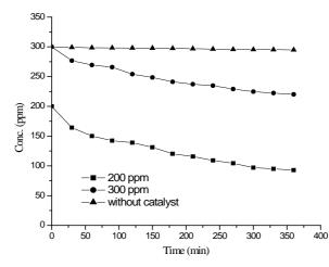
Fig. 7. Effect of initial solution concentration on photodegradation of RY at constant layer thickness in continuous mode. ( $C_0 = 200$ , 300 ppm; Catalyst dose = 5 g TiO<sub>2</sub> /5 g cement; Operation time = 360 min;  $T = 40^{\circ}$ C; Solution layer thickness = 3.7 mm; Flow rate = 1 mL/min.)
