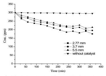
Fig. 4. Effect of solution depth on photodegradation. ( $C_0 = 300$ ; Catalyst dose = 5 g TiO<sub>2</sub> /5 g cement; Operation time = 360 min;  $T = 40^{\circ}$ C; Solution layer thickness = 2.77, 3.7, 5.5 mm)
