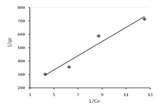
Fig. 2. Langmuir isotherm "Eq. (1)" plot for RY adsorption onto TiO<sub>2</sub> plate. (Adsorbent dose = 50 kg/m<sup>3</sup>; Temperature =  $26\pm 2^{\circ}$ C, Initial RY concentration,  $C_{o} = 150, 200, 300, 400$  ppm).
