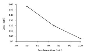
Fig. 6. Effect of residence time on photodegradation of RY at constant initial concentration in continuous mode. ( $C_0 = 200$  ppm; Catalyst dose = 5 g TiO<sub>2</sub> /5 g cement; Operation time = 360 min;  $T = 40^{\circ}$ C; Residence time = 50, 75, 100 min; Flow rate = 1 mLO/min.)
