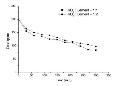
Fig. 9 Effect of catalyst dosage in photo-catalytic plate on RY degradation. ( $C_0 = 200$  ppm; Catalyst dose = 5 g TiO<sub>2</sub> /5 g cement, 5 g TiO<sub>2</sub> /10 g cement ; Operation time = 300 min;  $T = 40^{\circ}$ C; Solution layer thickness = 3.7 mm)
