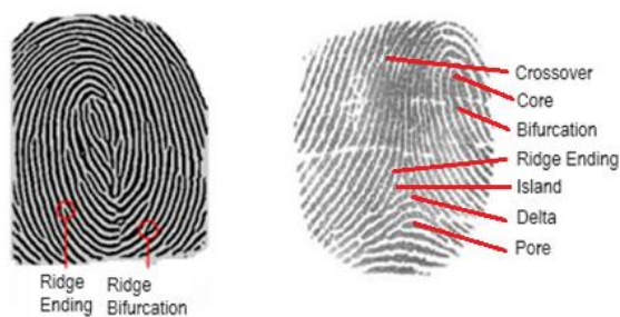
Fig. 1. Important feature like minutiae and their characteristics in a given fingerprint 2 .
