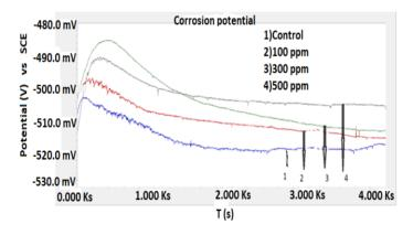
Fig. 2. Open circuit potential of mild steel without and with different concentrations of metronidazole (MNZ) in *Barr's* medium inoculated with SRB.
