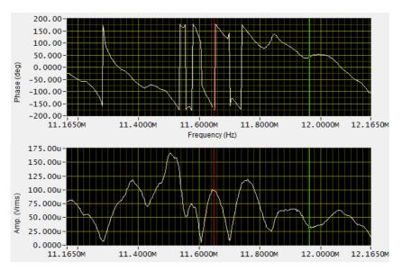
Fig. 5. Screenshot saved by HF2 LIA zi control interface at 760 Torr: 760 torr resonance is found using the HF2 LIA zi control screen by monitoring the resonance at 0 dBm driving power and detecting resonance at each decade of pressure, as shown in Fig. 4. Both amplitude and phase responses can be monitored simultaneously on the screen. The red line on the screen indicates the maximum amplitude of mechanical resonance where the phase slope is the steepest.
