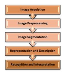
Fig. 1. Phases of image processing.
