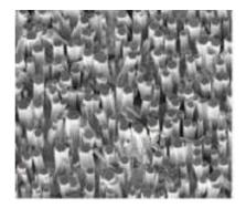
Fig. 4. SEM image of the as-synthesized ZnO NWs a chemical approach [2].
