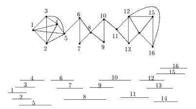
Fig. 1. An Interval graph with its interval representation.
