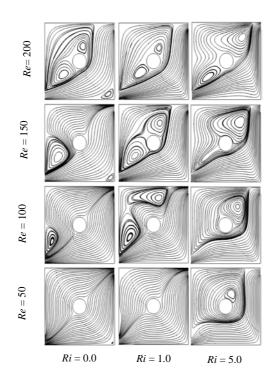
Fig. 2. Streamlines for various Reynolds numbers and Ri, while Pr = 0.71.
