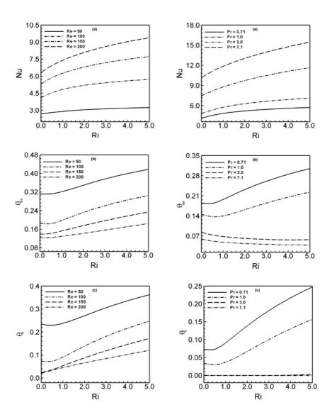
Fig. 6. Effect of Re on (a) average Nusselt number, (b) average fluid temperature and (c) temperature at the cylinder center in the cavity, while Pr = 0.71.
