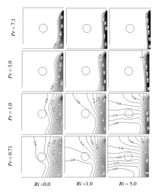
Fig.5. Isotherms for different values of Prandtl numbers and Ri, while Re = 100.
