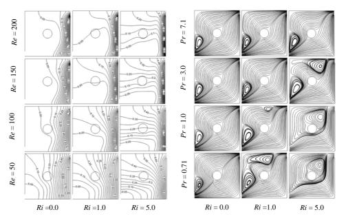
Fig. 3. Isotherms for various Reynolds numbers and Ri, while Pr = 0.71.
