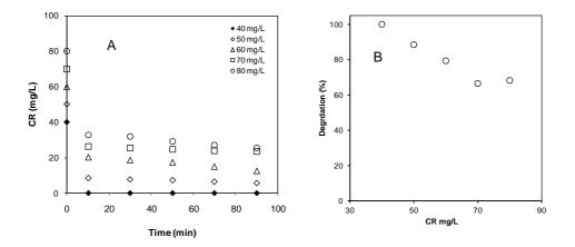
Fig. 4. A) Irradiation time dependent concentration variation for the photodegradation of CR having different initial concentrations in presence of fixed dose (0.05 g) of NiO/SiO<sub>2</sub>/PGMA nanocomposite particles. B) Percentage of degradation at different initial concentrations of CR in presence of fixed dose (0.05 g) of NiO/SiO<sub>2</sub>/PGMA nanocomposite particles. Conditions: pH 7; temperature, 30°C; total volume, 50 mL.
