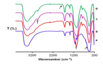
Fig. 1. FTIR spectra of a) NiO nanoparticles, b) NiO/SiO<sub>2</sub> and NiO/SiO<sub>2</sub>/PGMA nanocomposite particles (c, d) prepared with different NiO/SiO<sub>2</sub> to PGMA ratios: c) 1/0.5 and d) 1/1.
