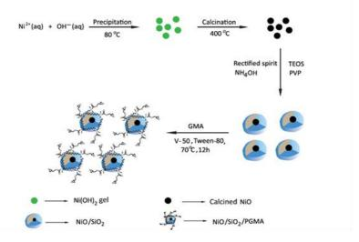
Scheme 1. Reaction scheme for the preparation of NiO/SiO2/PGMA nanocomposite particles.
