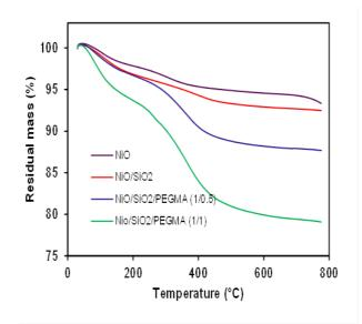
Fig. 3. TGA thermograms of NiO nanoparticles, NiO/SiO<sub>2</sub> and NiO/SiO<sub>2</sub>/PGMA nanocomposite particles.
