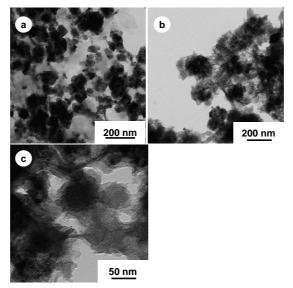
Fig. 2. TEM images of (a) NiO nanoparticles, (b)  $NiO/SiO_2$  and (c)  $NiO/SiO_2/PGMA$  nanocomposite particles.
