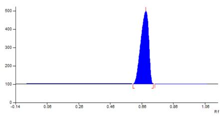
Fig. 2. Thin-layer chromatogram obtained from sinapic acid standard.
