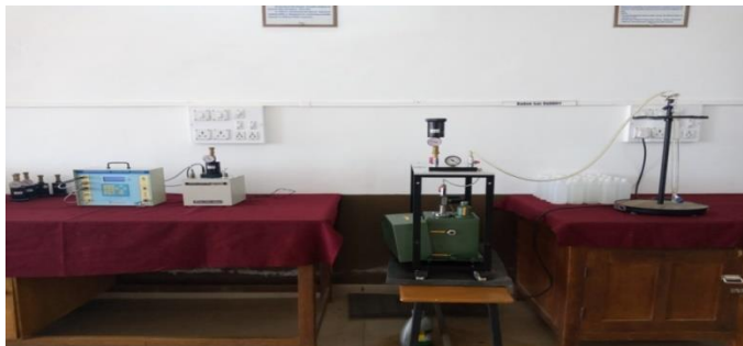
Fig. 2. Complete set up of Radon bubbler method.
