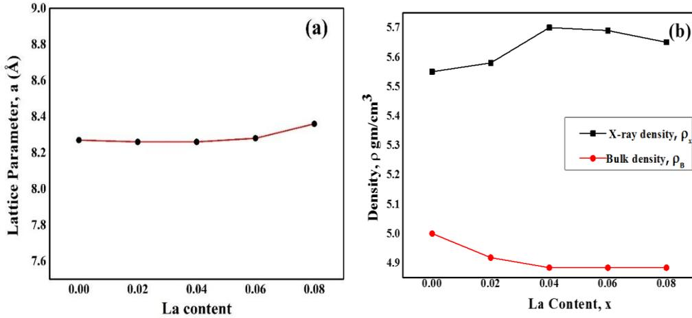
Fig. 2. Variation of (a) lattice parameter and (b) X-ray density and bulk density of  $Cu_{0.15}Zn_{0.85}La_xFe_{2-x}O_4$  as a function of La content.
