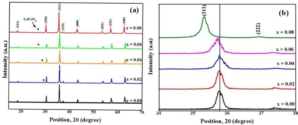
Fig. 1. (a) XRD pattern of  $\text{Cu}_{0.15}\text{Zn}_{0.85}\text{La}_x\text{Fe}_{2-x}\text{O}_4$ ; (b) Shifting of XRD plane for (311).
