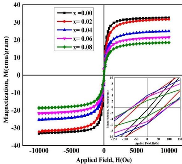
Fig. 4. Hysteresis loops (M-H curve) of  $Cu_{0.15}Zn_{0.85}La_xFe_{2-x}O_4$ , [ $x = 0.00, 0.02, 0.04, 0.06$  and  $0.08$ ].
