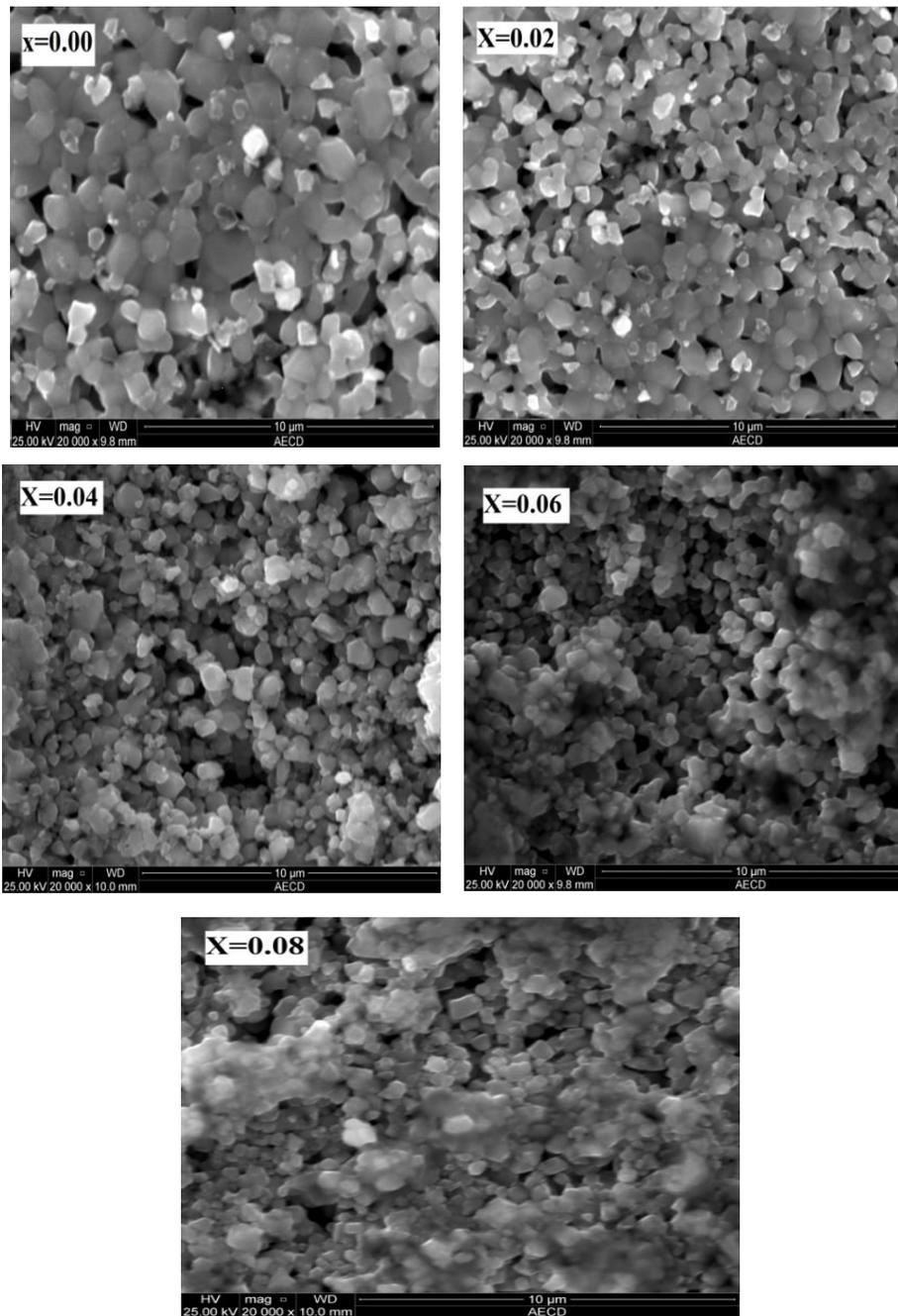
Fig. 3. SEM micrographs of  $\text{Cu}_{0.15}\text{Zn}_{0.85}\text{La}_x\text{Fe}_{2-x}\text{O}_4$ , [ $x = 0.00, 0.02, 0.04, 0.06$  and  $0.08$ ].
