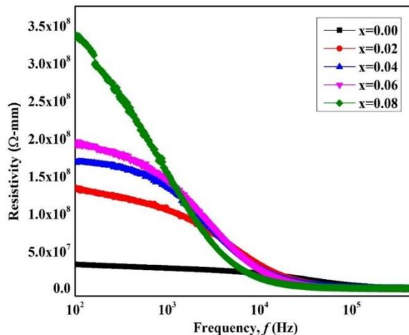
Fig. 5. Variation of the frequency dependent resistivity of  $\text{Cu}_{0.15}\text{Zn}_{0.85}\text{La}_x\text{Fe}_{2-x}\text{O}_4$ , [ $x = 0.00, 0.02, 0.04, 0.06$  and  $0.08$ ].
