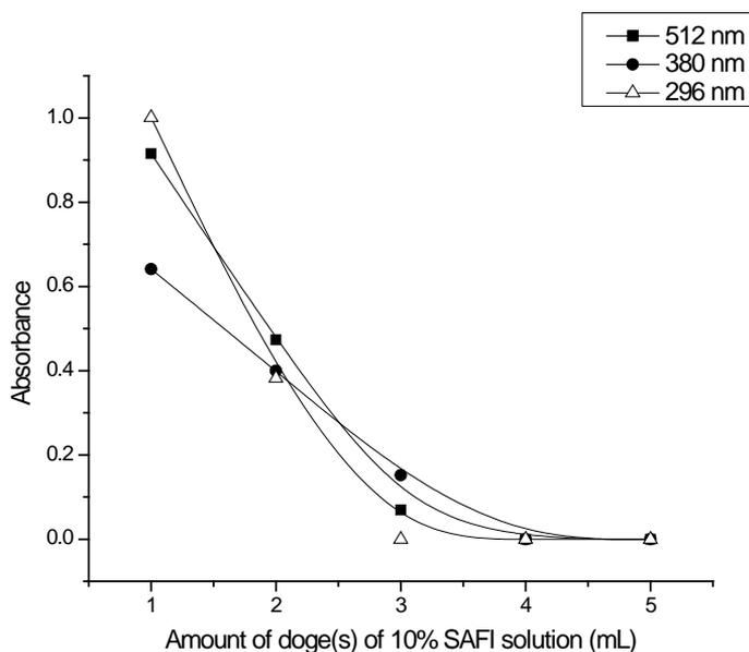
Fig. 4. Variation of absorbance with different dosages of SAFI solution at pH 7.
