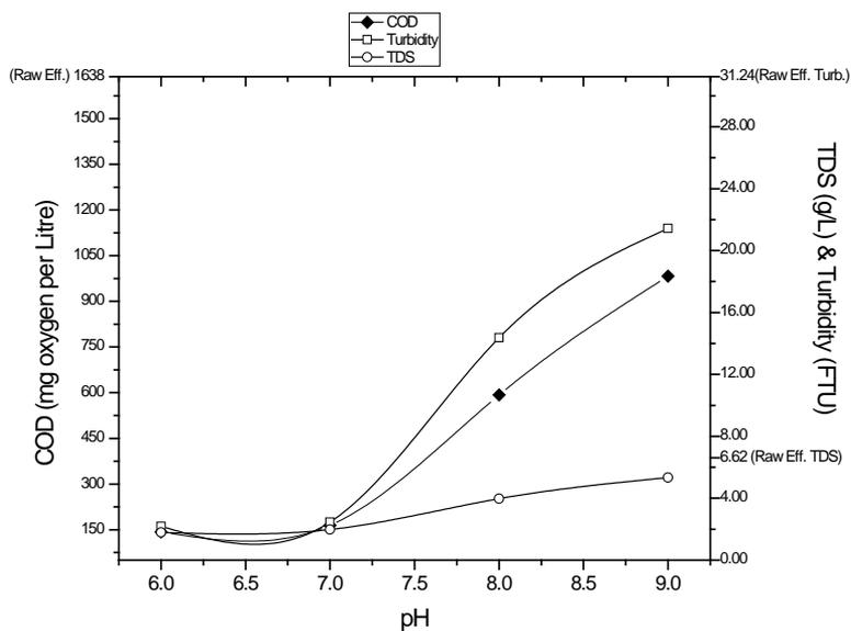
Fig. 5. Treatment of the effluent in terms of COD, TDS and Turbidity using SAFI solution as a function of pH.
