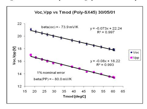
Figure 3: Open circuit and peak volatage graphs versus module temperature
