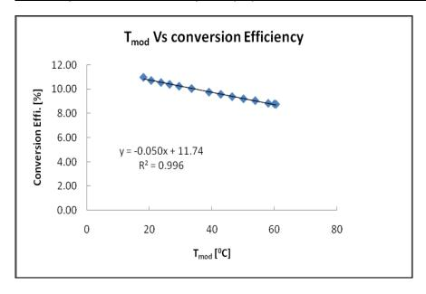
Figure 5: Efficiency graphs versus module temperature of the modules under investigation
