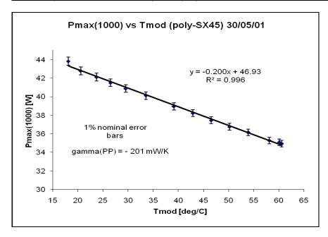
Figure 4: Maximum power graphs versus module temperature
