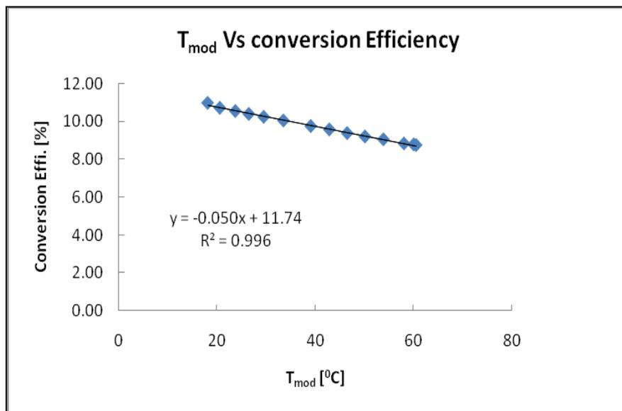
Figure 5: Efficiency graphs versus module temperature of the modules under investigation
