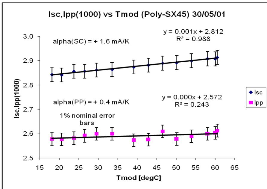
Figure 2: Short circuit and peak current graphs versus module temperature
