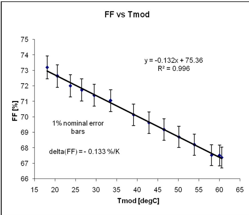
Figure 5: Fill factor graphs versus module temperature
