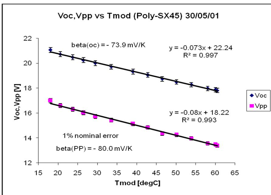
Figure 3: Open circuit and peak voltage graphs versus module temperature
