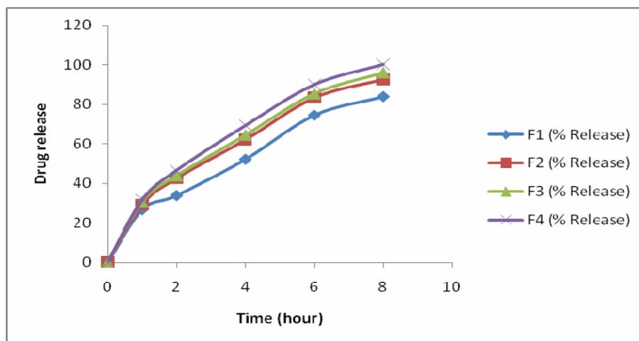
Figure 1. Zero order release profile of Methocel K100 LVCR based formulations containing PEG 6000.
