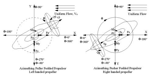
Figure 4: Definitions of forces, moments, coordinate of the puller and pusher azimuthing podded propulsors.
