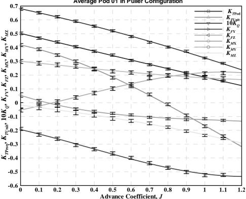
Open Water Propulsive Performance Curves with Error Bars Average Pod 01 in Puller Configuration
