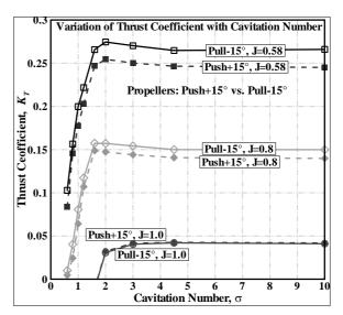
Figure 8: Comparison of thrust coefficient (Push+15° and Pull-15° propellers) variation with cavitation number for fixed advance coefficients.
