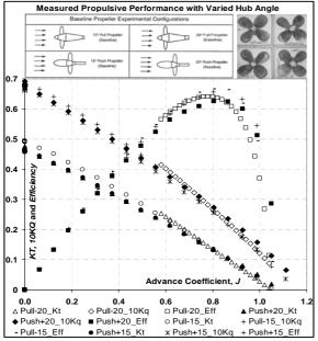
Figure 7: Performance characteristics of podded propeller (propeller only case) with four different hub taper angles.
