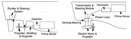
Figure 1: Conventional propulsion system (left) vs. podded propulsion system (right).
