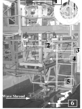
Figure 2: Different parts of the experimental apparatus used in the podded propulsor tests (MacNeill *et al.* 2004).
