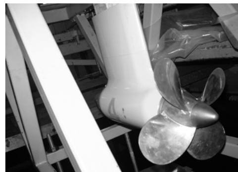
Figure 12: Pod 4 attached to the apparatus before being tested.
