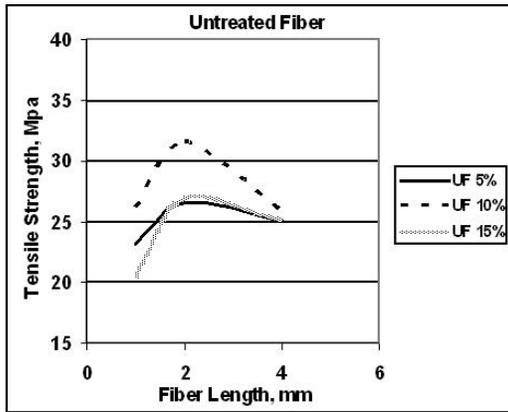
Fig. 3: Tensile Strength of Untreated Jute Fiber Composites at Different Lengths\*
