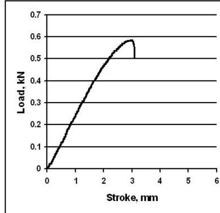
Fig. 2: An observed load-stroke curve obtained from tensile test
