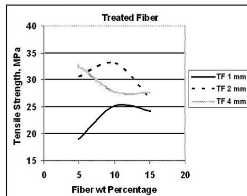
Fig. 6: Tensile Strength of Treated Jute Fiber Composites at Different Fiber wt. Percentages\*
