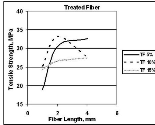
Fig. 4: Tensile Strength of Treated Jute Fiber Composites at Different Lengths\*
