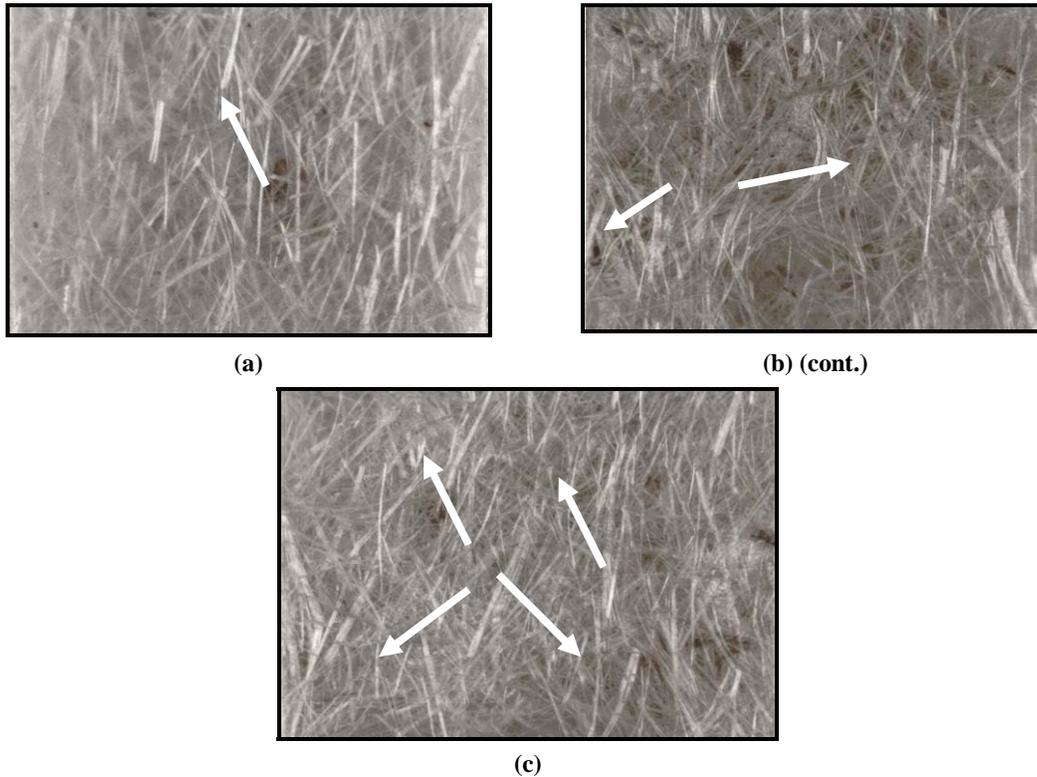
**Fig. 1:** Optical microscopy of jute fiber reinforced polymer composites reinforced with various fiber wt. percentages. (a) 5% Fiber (b) 10% Fiber (c) 15% Fiber. Entanglement of fibers is shown by the arrow. It is clear that 15% fiber composite has highest fiber entanglement compared to 5 & 10% fiber composites
