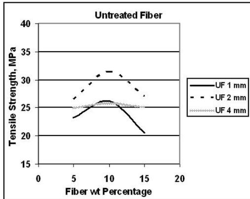
Fig. 5: Tensile Strength of Untreated Jute Composites at Different Fiber wt. Percentages\*
