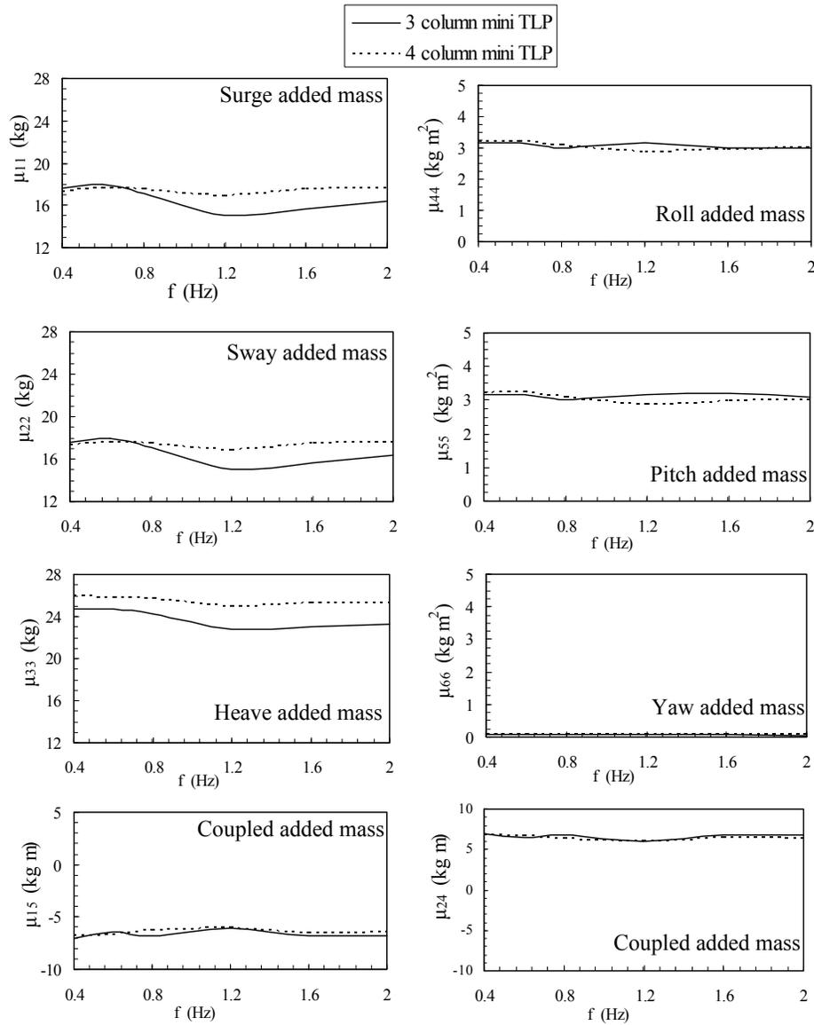
**Fig. 3.** Comparison of added mass of mini TLP models.
