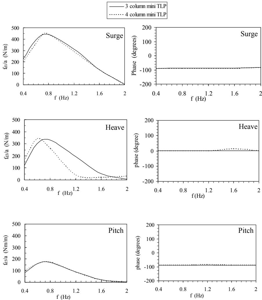
Fig. 5. Diffraction force components and their phases.
