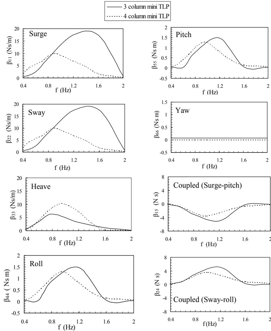
**Fig. 4.** Radiation damping coefficients of mini TLP models.
