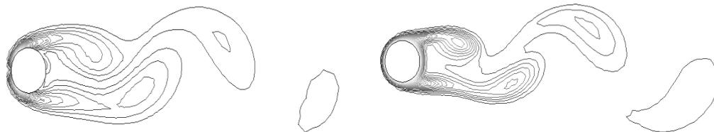
Fig.9: Instantaneous Vorticity (left) and Isotherm (right) at  $Re=100$ ,  $Ri=1$  and  $\phi=0.05$ .
