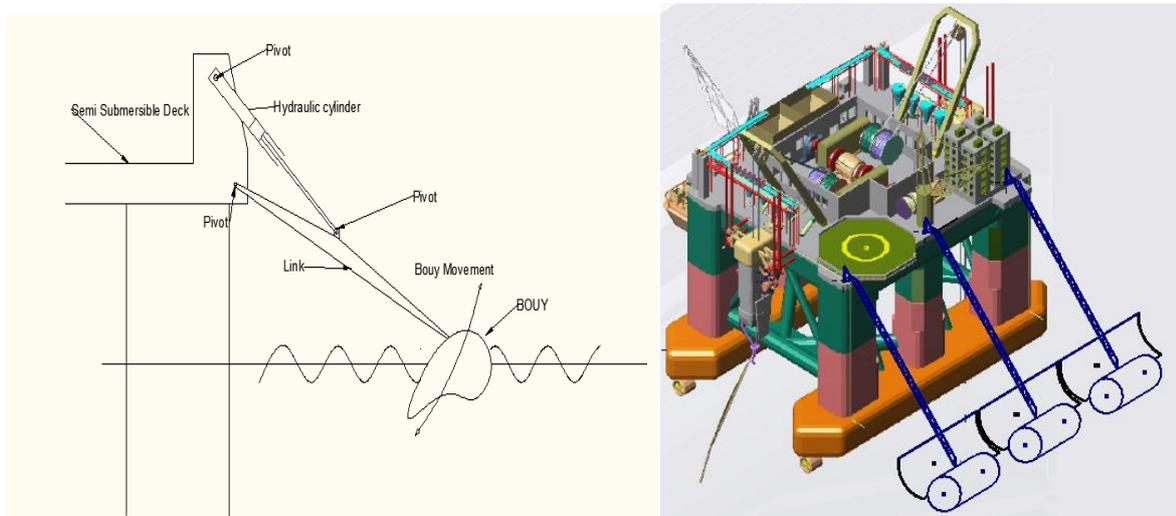
Fig. 1: Proposed deep ocean wave energy system (concept)
