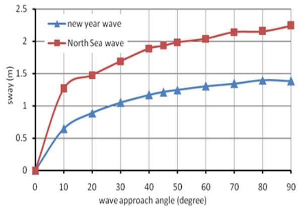
Fig. 7(b): Variation of the maximum response in sway degree-of-freedom
