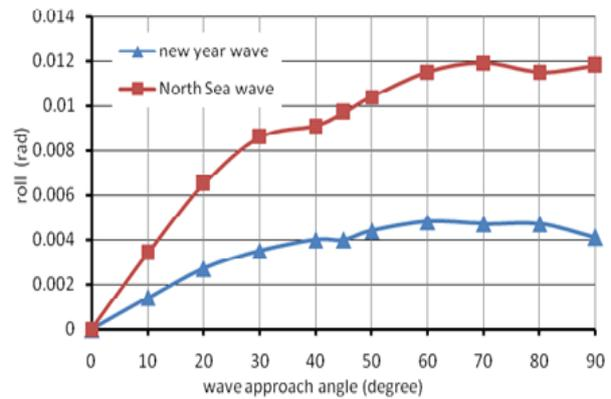
Fig. 7(d): Variation of the maximum response in roll degree-of-freedom
