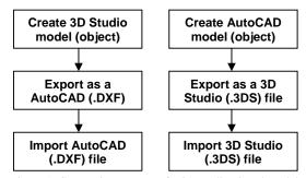
Figure 1: Conversion process of a 3D studio virtual model to an AutoCAD model (left) and that of an AutoCAD model to a 3D studio Virtual model (right).
