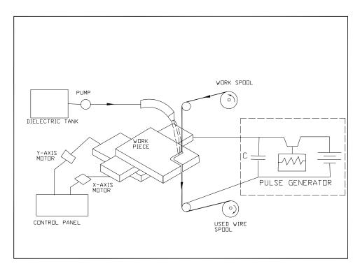
Figure 1. Schematic view of Wire cut EDM
