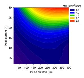
Figure 2. 2-D contour plot of the effect of peak current and pulse on time on MRR.
