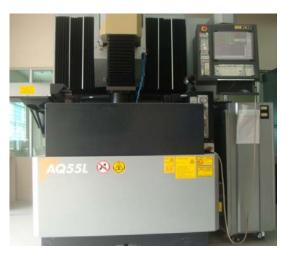
(a) Photograph of the EDM at machining
