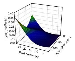
Figure 9. 3-D surface plot of the effect of peak current and pulse on time on TWR.
