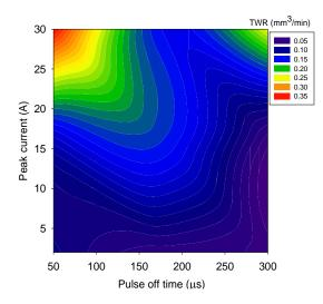
Figure 8. 2-D contour plot of the effect of peak current and pulse off time on TWR.
