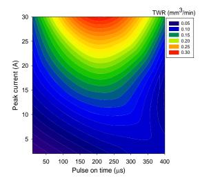
Figure 6. 2-D contour plot of the effect of peak current and pulse on time on TWR.
