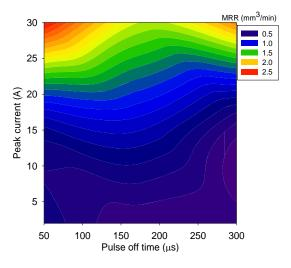
Figure 4. 2-D contour plot of the effect of peak current and pulse off time on MRR.
