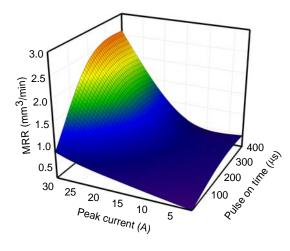
Figure 3. 3-D surface plot of the effect of peak current and pulse on time on MRR.
