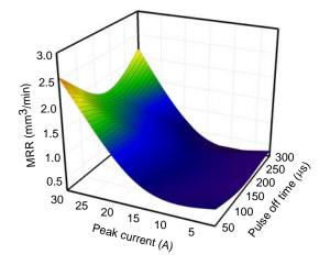
Figure 5. 3-D surface plot of the effect of peak current and pulse off time on MRR.
