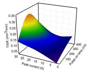
Figure 7. 3–D surface plot of the effect of peak current and pulse on time on TWR.
