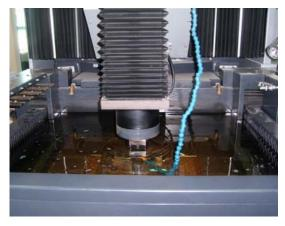
b) Photograph of the EDM tank and sample at operational condition.
