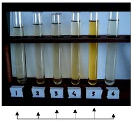
Figure 3(a). Colour comparison of petrol samples, arrow sizes indicate colour darkness.
