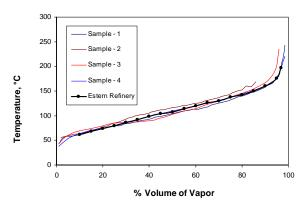
Figure 8(b). Distillation curve of Octane samples.
