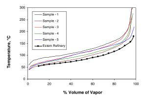
Figure 8(a). Distillation curve of Petrol samples.
