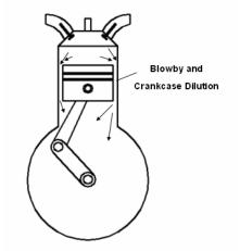
Figure 1. Crankcase dilution inside the engine
