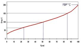
Figure 6. Typical distillation curve for gasoline.
