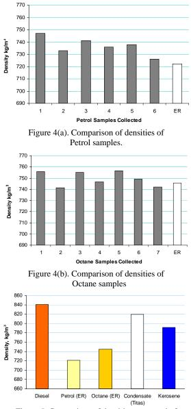
Figure 5. Comparison of densities measured of different types of colour coded fuels.
