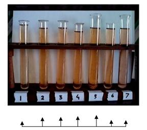
Figure 3(b). Colour comparison of octane samples, arrow sizes indicate colour darkness.
