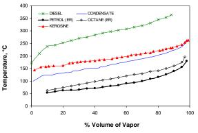
Figure 9(a). Distillation curve of different fuels samples.
