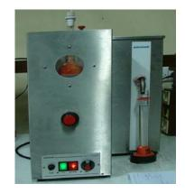
Figure 7. Distillation-Unit used, DU-4 Professional
