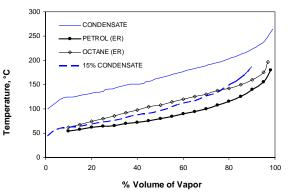
Figure 9(b). Distillation curve of 15% Condensate by volume with Petrol.
