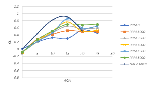
Figure 10. Effect of leading edge rotating cylinder on the lift and stall characteristics of NACA 0018 at various RPM at V= 30 m/s.
