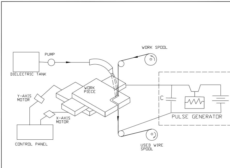
Figure 1. Schematic view of Wire cut EDM
