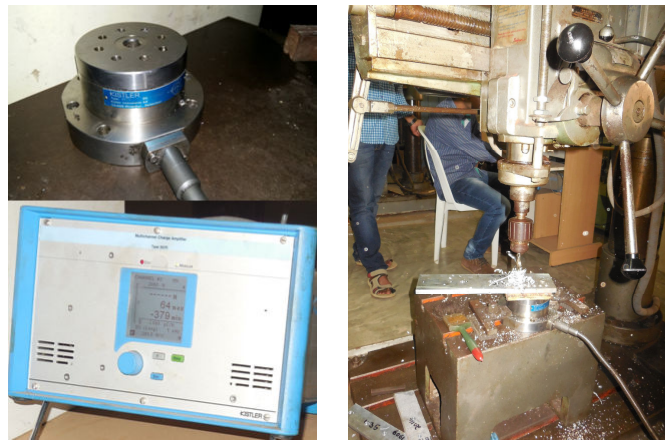
Figure 1. Kistler dynamometer type 9272 (Kistler Instrumente AG, CH8408 Winterthur, Switzerland), Multichannel signal amplifier (kistler type 5070) and radial drilling machine (Make: Siddapura Machine Tools, Gujarat, INDIA).
