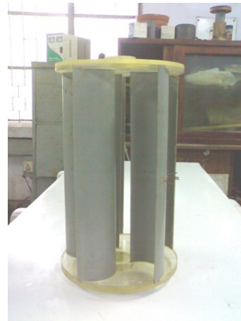
Figure 2: Five bladed vertical axis vane type rotor.
