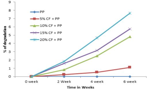
Fig. 2. Degradation of CF+PP composites in soil.
