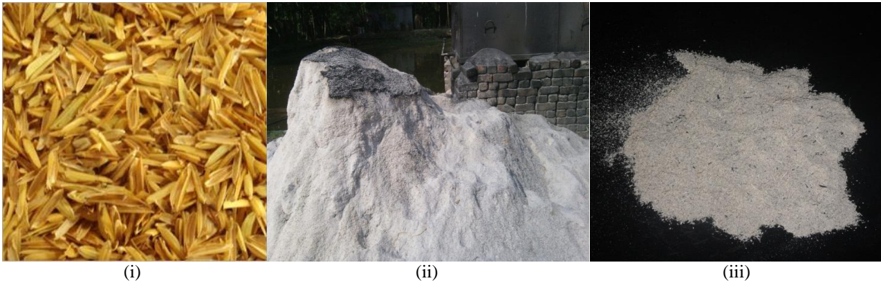
Fig. 1. (i) Rice husk before burning, (ii) Waste RHA after burning at a rice mill (iii) RHA for use in concrete
